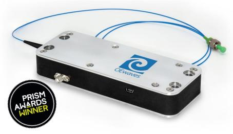
This HI-Q™ laser houses a proprietary driver/controller and the OEwaves laser source which is based on a high quality factor (Q) Whispering Gallery Mode (WGM) micro-resonator. The laser is available at a variety of C band wavelengths (1530 – 1565 nm).
