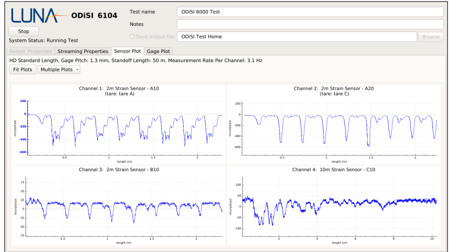
Multichannel sensor plot (strain/temperature versus length) in the ODiSI software.
