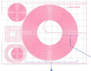
For example, the Optoelectronics Research Group at UCSB fabricated a one meter spiral delay line on a silicon platform. The OBR 4600 was used to measure the distributed loss inside the photonic integrated circuit (PIC), which measured only 1 cm<sup>2</sup> in size.
