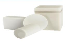
slightly over the spectrum (see Figure 1). Similarly, carbon black is used as a universal absorbing dye providing a mostly flat absorption coefficient ( $\mu$ a) as a function of wavelength (see Figure 2). Thus, every phantom fabricated has its own absorption and scattering characteristics.
