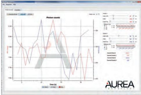
A user-friendly Graphical User Interface is provided. It allows the set-up of the QE, gate width, delays, deadtime, and also the display of the photon count, the clock, the temperature and the alarm to protect against accidental overload. The DLL libraries compatible to the most well-known programming languages are also provided.
