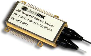
Accelink’s integrated coherent receiver integrates signal polarization beam splitter, two optical 90° hybrids, four sets of high speed balanced photodiodes and four differential linear amplifiers in a single compact surface-mount package. The device demodulates the state-of-polarization and optical phase of a phase-modulated signal relative to an externally supplied optical reference, enabling recovery of the 100 G/s Dual Polarization Quadrature Phase Shift Keyed (DP-QPSK) format signals.
