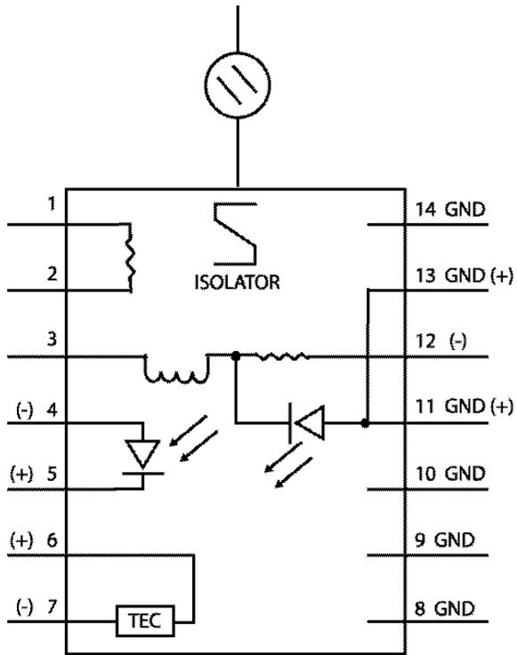
Figure 1. Laser Schematic
