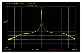
In this measurement the spectral shape of a DFB laser is shown. Even without applying any modulation, the laser own intensity noise modulates it, showing its intrinsic response and revealing its potential bandwidth. Also, just by measuring the spectral linewidth at different bias currents the linewidth enhancement factor can be extracted.
