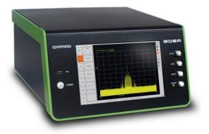
Its simultaneous 10 MHz (80 fm) resolution and 80 dB spurious-free dynamic range, make the BOSA200 the best performing high-resolution OSA. The non-linear nature of SBS creates a filter that is not only narrow but extremely sharp, maintaining a width under 1 pm more than 50 dB below the peak, which allows for precise measurement of signal components even really close to the optical carrier.
