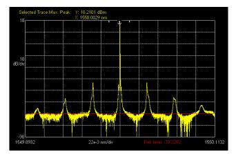
In the above measurement example, the spectrum of a narrow external cavity laser is shown. Thanks to its dynamic range and **absence of artifacts**, the BOSA reveals the true spectral shape of the laser, whereas in heterodyne OSAs the spectral shape of the local oscillator will be imprinted in all the spectrum distorting the measurement.
