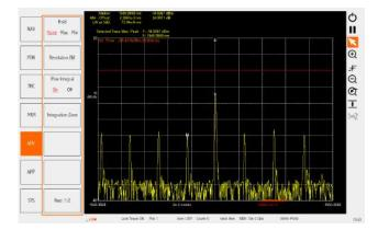
Dual-channel polarization measurement, that allow seeing the separate orthogonal polarization components of the signal simultaneously.
