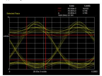
For phase measurements, only the I and Q eye diagrams can be measured as they require demodulation. However, as BOSAphase performs its measurement with **no need for demodulation**, the real phase eye diagram can be obtained. This allows as shown in the example measurement below, rendering the **multi-level phase eye diagram** of a QPSK modulation.
