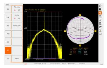
This enables real-time measurement of the instantaneous differential group delay (DGD) of the channels present in an in-service DWDM link. By monitoring DGD over time, polarization mode dispersion (PMD) of the fiber can be measured.
