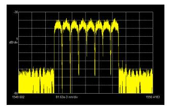
In the example below, an upconverted OFDM signal after optimizing the ADC stage thanks to the information obtained by BOSA. Seeing the spectral shape is critical!
