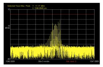
BOSA is also a great tool to analyze dynamic effects on lasers and semiconductor devices. In the measurement examples above and below we can observe a close-up of a Fabry Perot mode which is directly modulation with a 500 MHz tone and a picosecond pulsed laser with a 10 GHz repetition rate.
