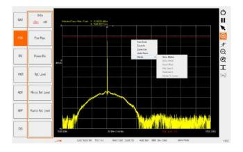
BOSA graphic user interface has been completely redesigned to be fast and operative either through its included **touch screen** (with big clear buttons, ideal for use when mounted in a rack) or with **mouse and keyboard** and external monitor (getting advantage of shortcuts and contextual menus, great when installed in a lab workbench or in a cart).
